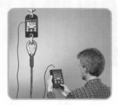
When the TL6000 is configured with a display, the TL-IND2 and TL-RF2 remote indicators provide a tandem display capability as well as On/Off, Tare and Zero functions.
